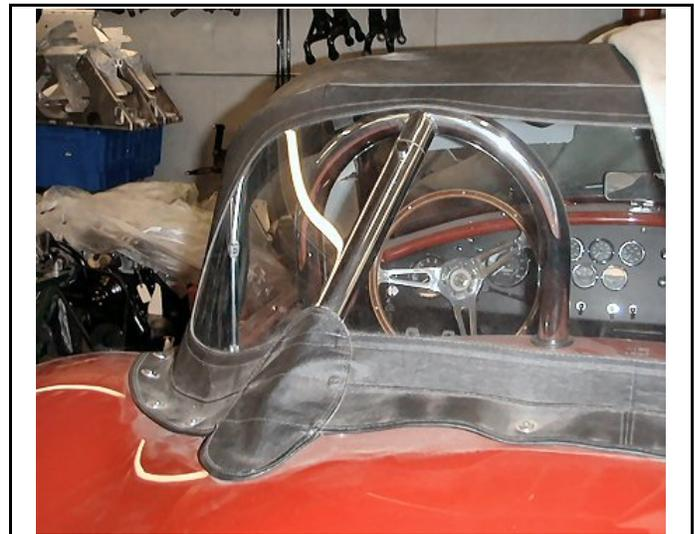
Beginning at the center, carefully un-tape a portion of the top fabric from the windshield. Glue a portion of the top fabric to the front vertical face of the channel with contact cement. Do not apply the glue to the top of the front bow, only to the front surface. Work from the center to the sides until the entire top surface is glued.
