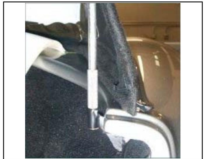
Assemble the rear bow halves together. Turn the knurled adjusters all the way into the ends of the bows.
