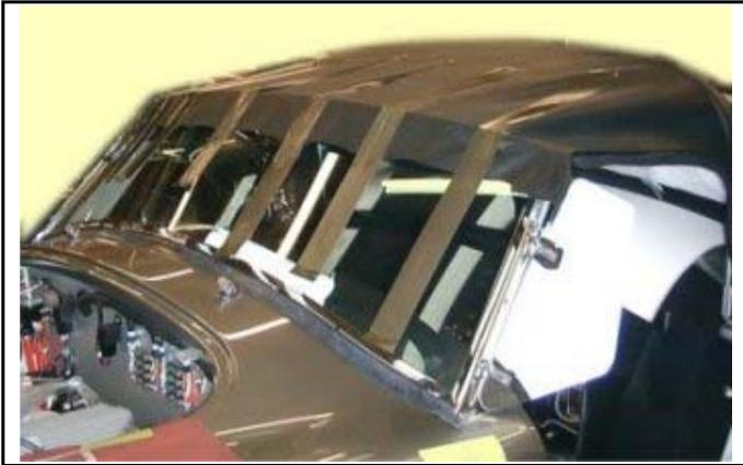
Alternately adjust the top over the rear bows and pull and re-tape the top material at the front to remove slack from the top and minimize wrinkling. Do not pull hard at any time. Stress can break the windshield! Make sure the top material is centered on the front bows and windshield. Keep adjusting the fabric at the rear and front of car until the top is smooth and sag free.
