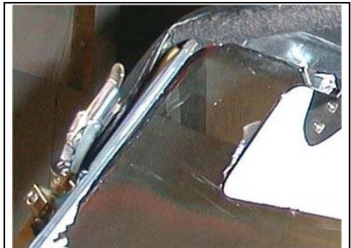
Secure the stationary brackets to the windshield side posts with the screws provided. Use a mild threadlocker like Loctite Blue on the screw threads.
