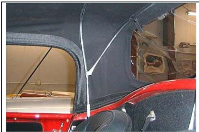
Install a snap on each rear flap as close as possible to the outside corner:
