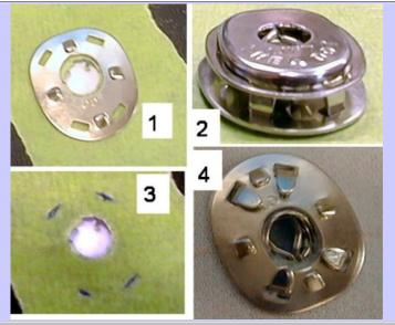
Locate the bottom stud. Drill a 1/8" hole and install the snap up into the floor. If the floor carpet is already installed, be careful that you don't drill too far. The carpet fabric may become entangled in the drill bit tangs.
