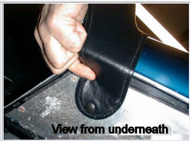
Check the fit onto the body curve. If it's OK, remove the protective tape from the back of the Velcro.
